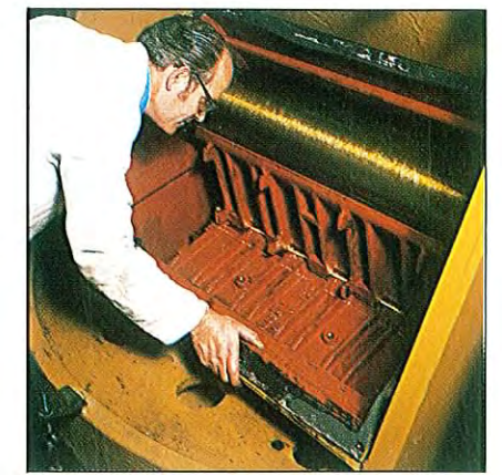
Toggles, pitman and eccentric operate in a sealed chamber . . .
