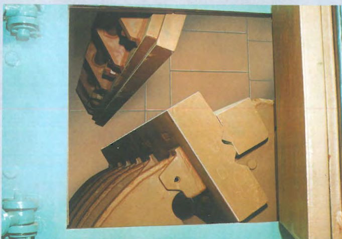
Crushing chamber with rotor-mounted blow bar and impact apron
