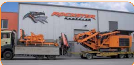
Transport - Screenbox splitted from machine
